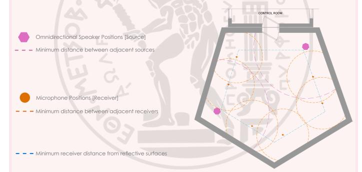
As depicted from the drawing above, an omnidirectional source (dodecahedron speaker) and a point receiver (microphone) were placed into the reverberation chamber in order to achieve a combination of 12 measuring positions as directed by the ISO 354:2003. The measurements were executed in 1/3 octave band analysis (Lz Weighting) follwing the precision method.
